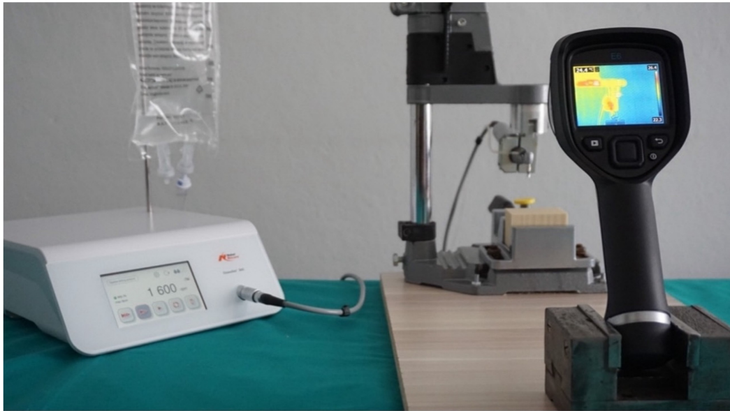
Figure 2. Experimental setup for measuring temperature changes during implant osteotomies.
