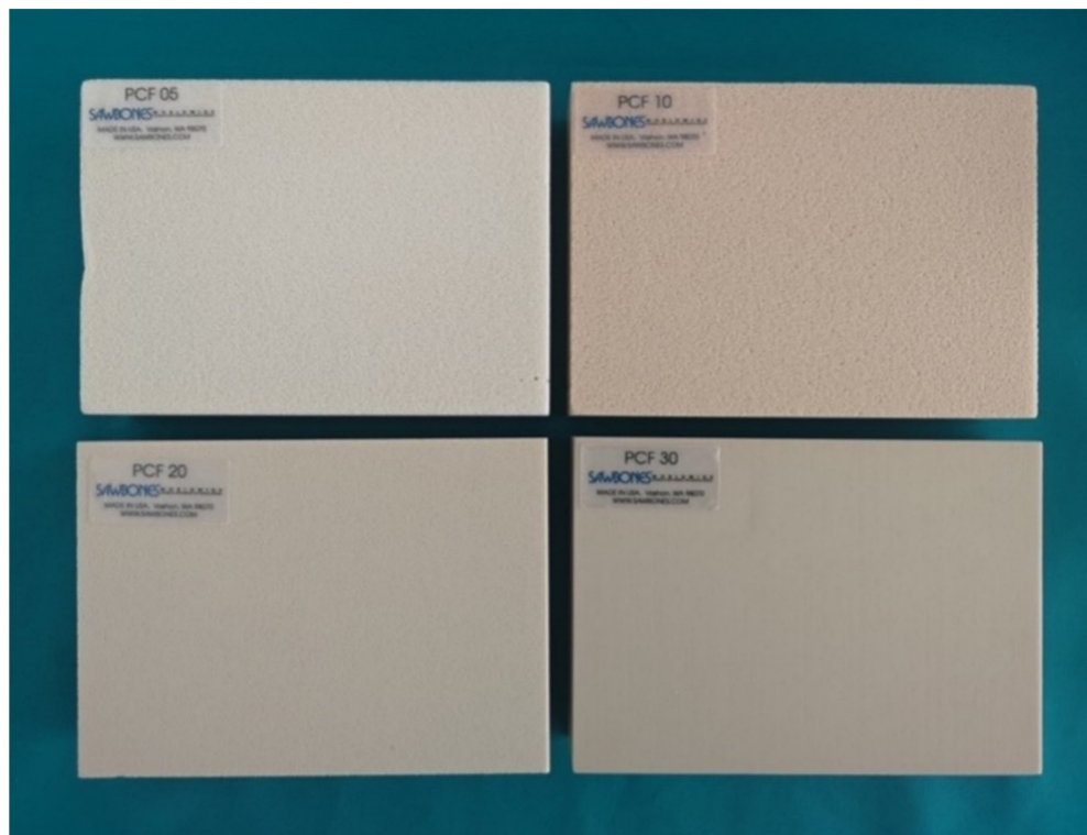
Figure 1. Artificial bone blocks of four different densities (D1–D4).
