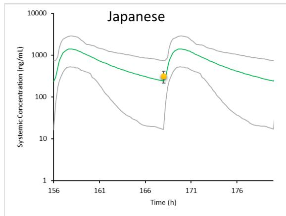
**Green lines represent the predicted mean; gray lines represent the predicted 5<sup>th</sup> and 95<sup>th</sup> percentile; orange circle and error bar represent the observed mean and standard deviation.**
